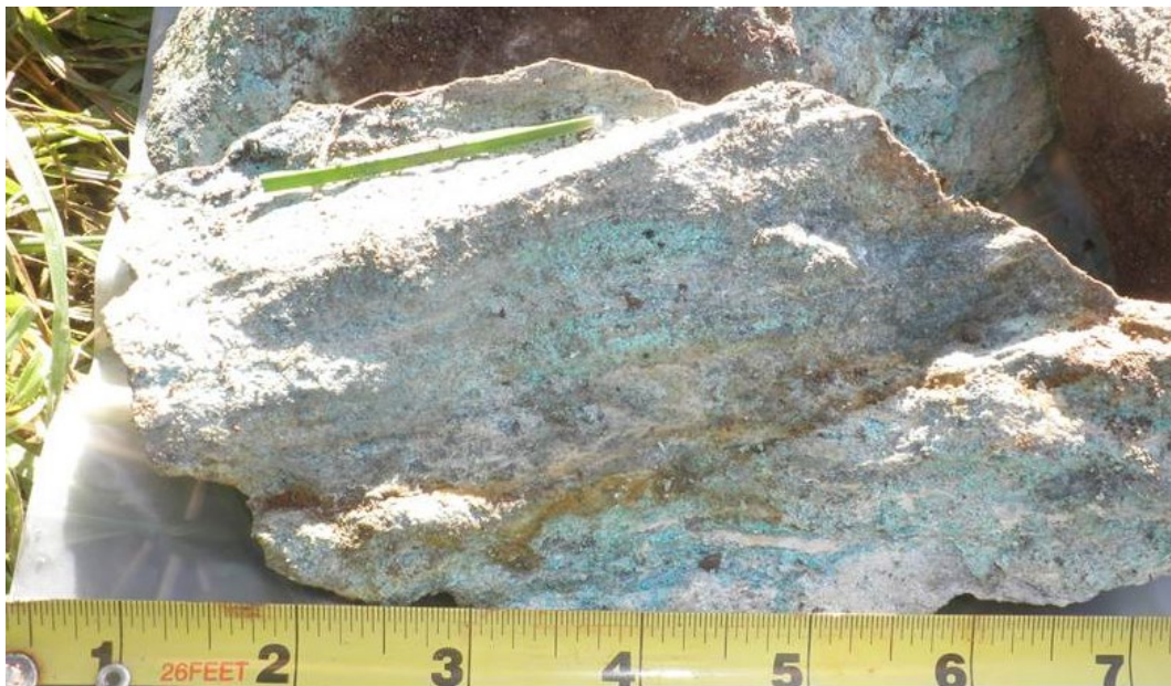
Disseminated bornite and secondary malachite in grey green sandstone float from wall at the Coosheen Mine area, West Carbery.
